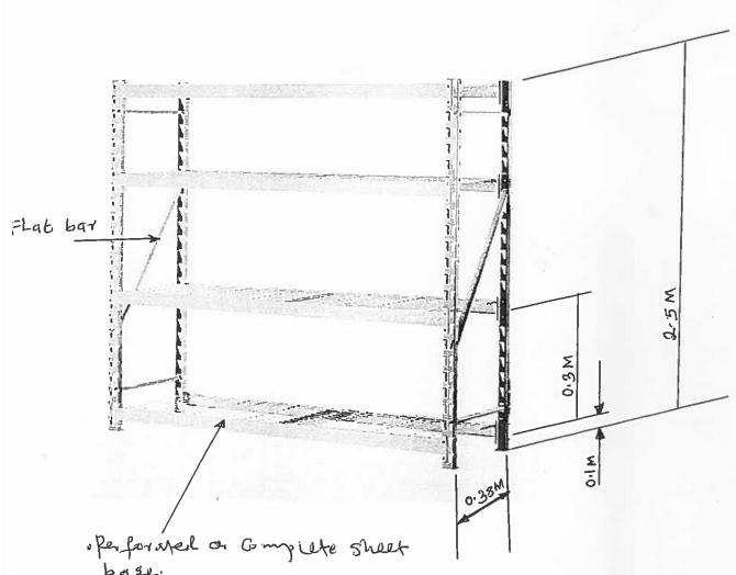
· Note: One side to be completely laveral by gauge 28 mild steel sheet size 1.5m x 2.5M.
